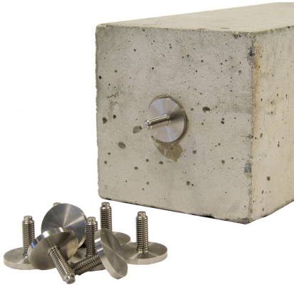
55-C0115/11. Steel pins to be glued on the beam ends surfaces
